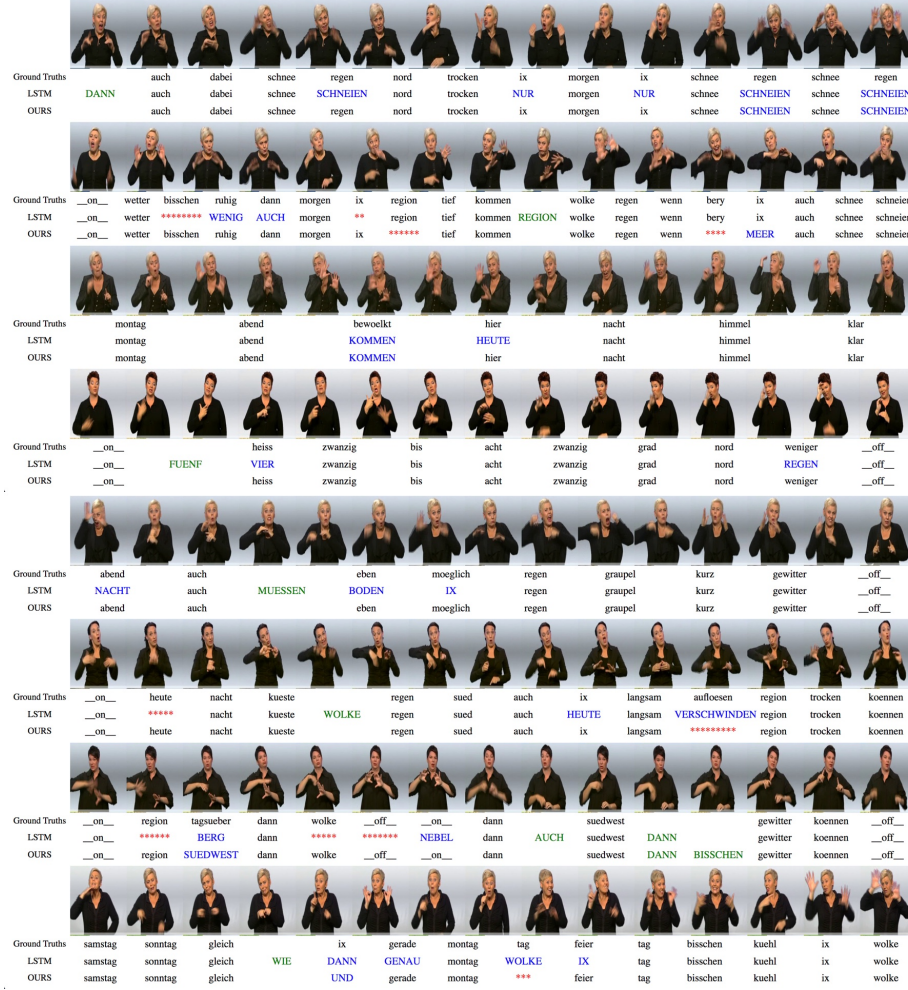
Fig. 1. Comparisons on full videos in the testing set of the RWTH dataset. Deletion, insertion, substitution errors are colored in red, green, blue, respectively. Glosses containing "___" are special flags that mark specific conditions in the signing sequences. "*****" represents missing glosses
