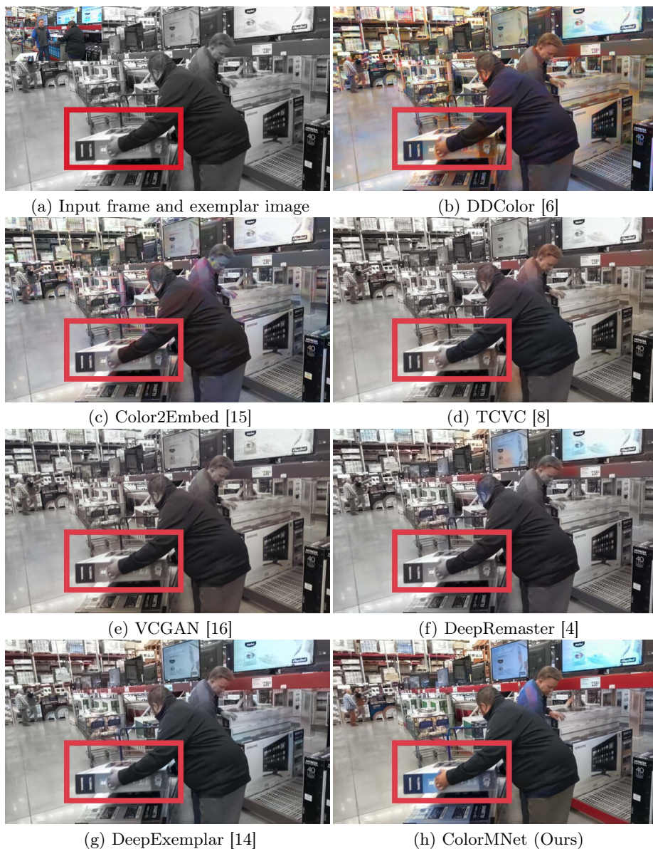
Fig. 9: Colorization results on clip loading from the DAVIS validation dataset [10]. The results shown in (b) and (c) still contain significant color-bleeding artifacts. In contrast, our proposed method generates a vivid and realistic frame, where the colors of the box and the man’s hands are better restored.
