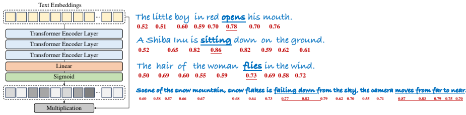
Fig. 3: Demonstrations for the structure of prompt adapter. We use three transformer encoder layers and a frame-specific linear layer to predict the weight of each text token. Examples are given on the right. In cases where multiple tokens correspond to a single word, we calculate the average weight for better visualization. The words with the maximum weight are underlined.
