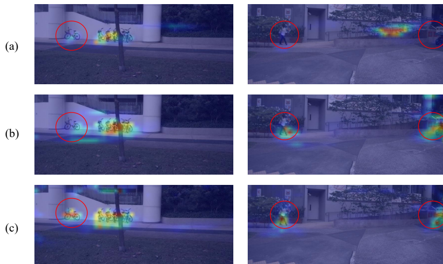
Fig. 5: Comparison of attention weight maps for the ray-aware position embedding of StreamPETR (a), the point-aware position embedding of 3DPPE (b), and the object-wise position embedding (c) on the nuScenes val set. After utilizing OPE, our OPEN can generate better attention weight maps for some hard-detected objects, which are highlighted by red circles.
