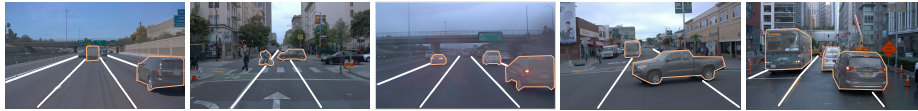
Fig. 1: Examples of road scenes, in which some lane parts are occluded by several objects. Visible lanes and obstructing objects are depicted by white lines and orange polygons, respectively.
