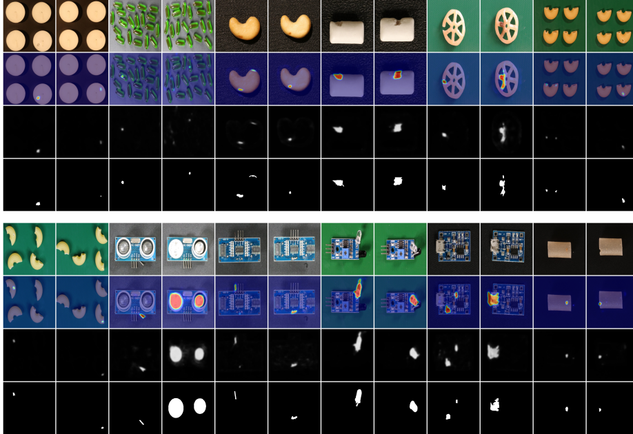
Fig. 4: Qualitative examples on VisA dataset. The original image, the anomaly map overlay, the anomaly map and the ground truth map are shown.
