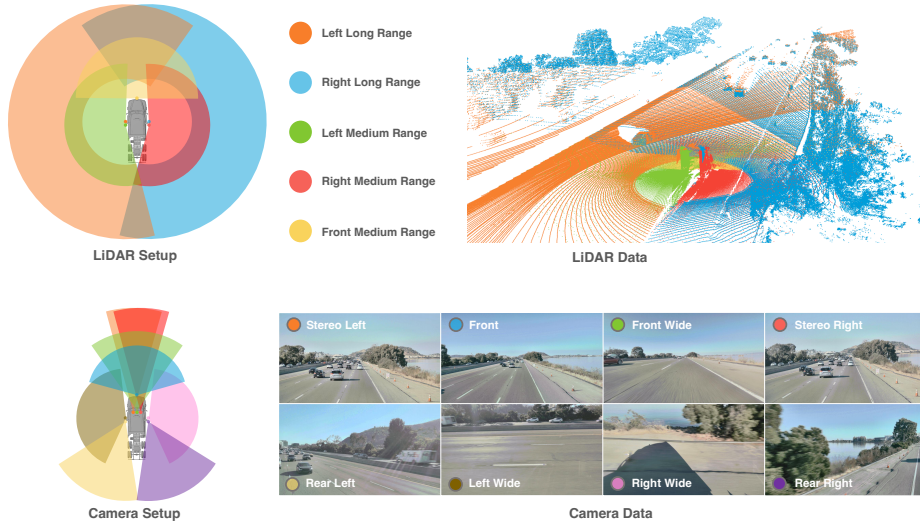
Fig. A2: MS-Cal dataset sensor setup and captured data. We show the LiDAR and camera data on the static outdoor collect.
