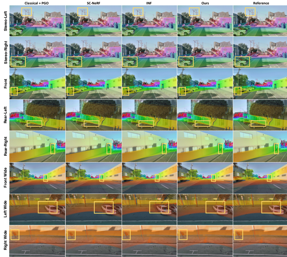
Fig. A6: More qualitative comparison on MS-Cal dataset. We show the projection of LiDAR and camera images for each camera sensor. Please zoom-in to see the mis-calibrations.
