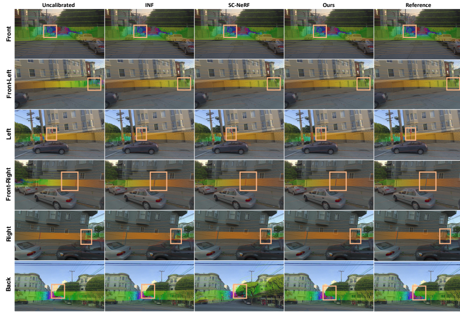
Fig. A4: More qualitative comparison on PandaSet dataset. We show the projection of LiDAR and camera images for each camera sensor. Please zoom-in to see the mis-calibrations.
