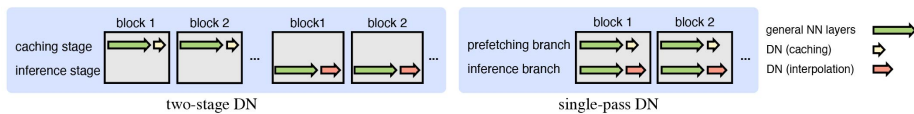
Fig. S4: Comparison of two-stage and single-pass DN. A naïve implementation of DN might resemble KIN, operating in two stages. However, our dispatcher design and prefetching strategy enable the prefetching branch to run in parallel with the inference branch across most neural network (NN) layers, and to execute asynchronously in the DN layer, effectively hiding the runtime of the prefetching branch.
