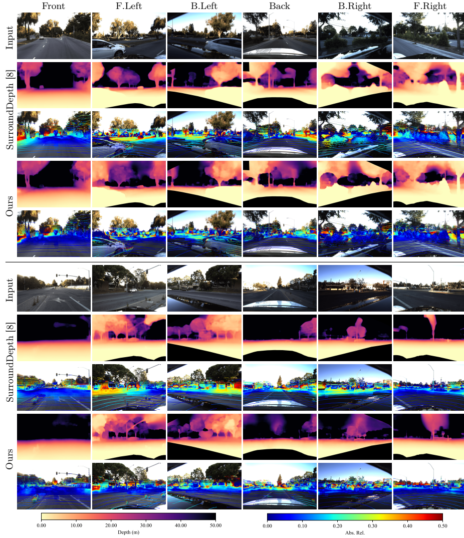
Fig. 6: Qualitative comparison of predicted surrounding depth on DDAD dataset [4]. Given the input surrounding images (the top row), we show the visualized depth maps and depth errors of SurroundDepth [8] and M^2 Depth. Our method is able to produce more accurate depth with less error and sharper depth edge across multiple cameras.
