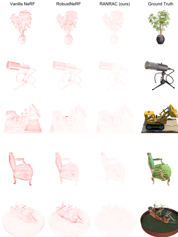
Fig. 10: Error visualization for scenes with blurred perspectives: We observe the global artifacts in the NeRF reconstruction and the local artifacts for view-dependent details in the RobustNeRF reconstructions indicated by a reddish highlighting (i.e., the larger the error the better visible it is in the difference image). In contrast, RANRAC does not produce global artifacts and has much lower prediction error for view-dependent details, solely caused by the scene representation itself.
